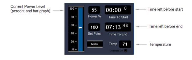
The main screen shows the current % power being output to the light fixtures, the time to start and time to end. In addition, the target power and room temperature are also shown.
