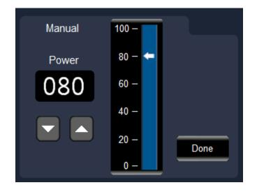
The manual mode allows the timed settings and max power to be adjusted in real time.
